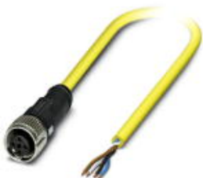
Sensor/actuator cable, 4-position, PVC, yellow, free cable end, on Socket straight M12 SPEEDCON, coding: A, cable length: 10 m
