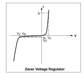
$\textbf{ELECTRICAL CHARACTERISTICS} \ (T_{A} = 25^{\circ}C \ unless \ otherwise \ noted, \ V_{F} = 0.9 \ V \ Max. \ @ \ I_{F} = 10 \ mA \ for \ all \ types)$
