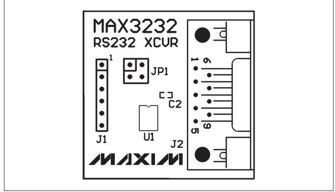
Figure 2. MAX3232PMB1 Peripheral Module Component Placement Guide—Component Side
