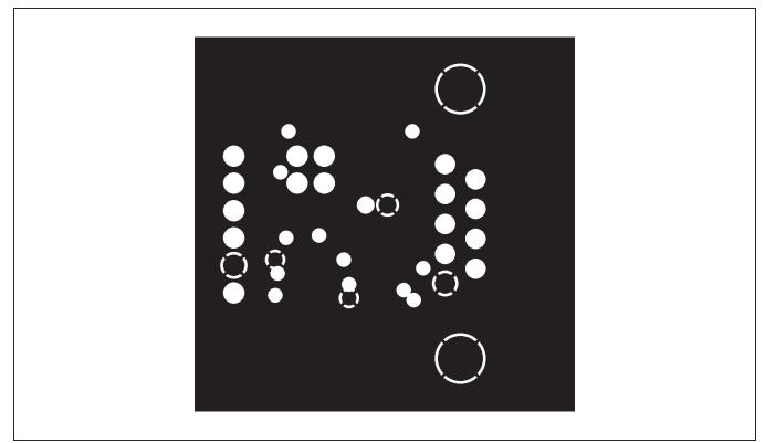
Figure 4. MAX3232PMB1 Peripheral Module PCB Layout—Inner Layer 1 (Power)
