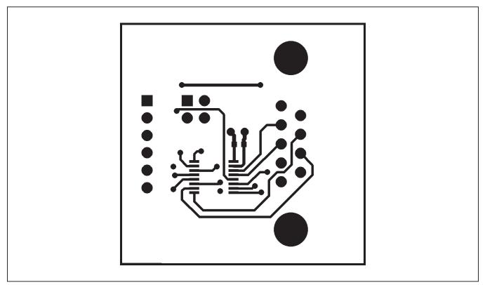
Figure 3. MAX3232PMB1 Peripheral Module PCB Layout—Component Side
