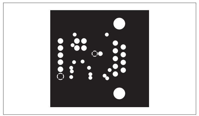
Figure 5. MAX3232PMB1 Peripheral Module PCB Layout—Inner Layer 2 (Ground)
