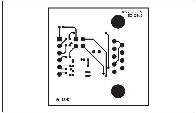
Figure 6. MAX3232PMB1 Peripheral Module PCB Layout—Solder Side
