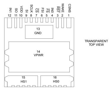
Figure 3. 33984 Pin Connections (Transparent Top View)
