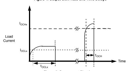
Figure 5. Overcurrent Shutdown
