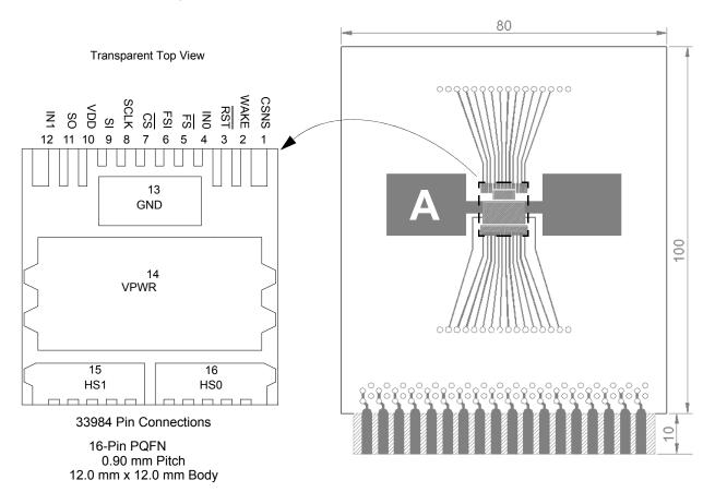
Figure 16. Thermal Test Board
