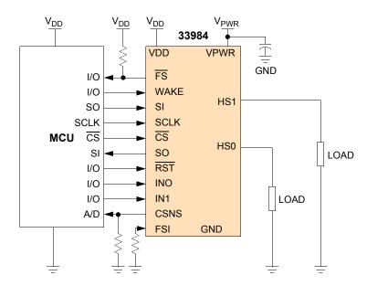
Figure 1. 33984 Simplified Application Diagram
