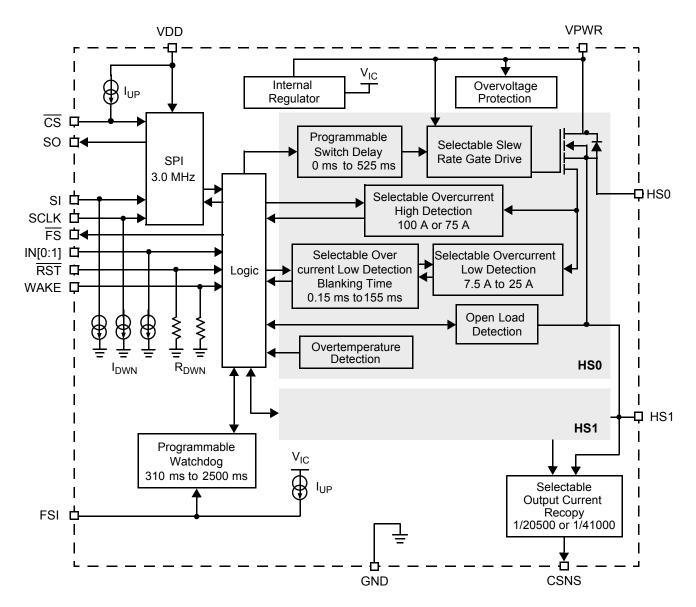
Figure 2. 33984 Simplified Internal Block Diagram
