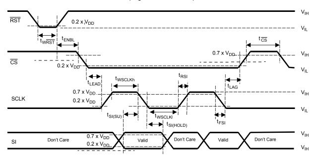
**Figure 7. Input Timing Switching Characteristics**
