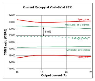
Figure 14. CSR0 Ratio Deviation in Function Manufacturing
