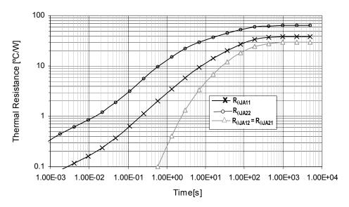
Figure 18. Transient Thermal Resistance  $R_{\theta JA}$  (1.0 W Step Response) Device on Thermal Test Board Area A = 600(mm²)
