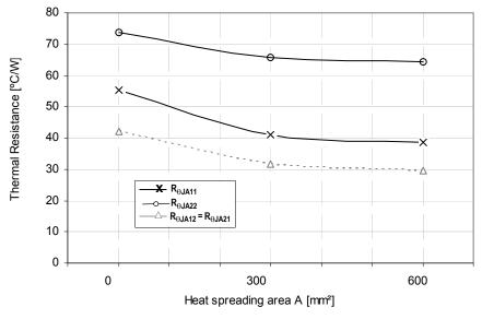
Figure 17. Device on Thermal Test Board  $R_{\theta JA}$
