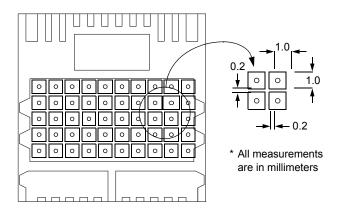
Note: Recommended via diameter is 0.5 mm. PTH (plated through hole) via must be plugged / filled with epoxy or solder mask in order to minimize void formation and to avoid any solder wicking into the via
