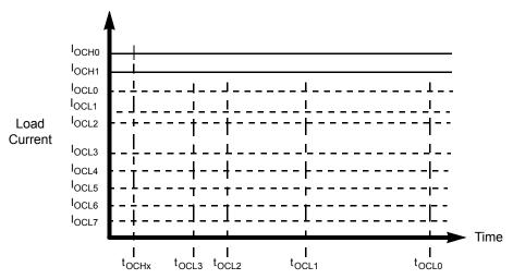
Figure 6. Overcurrent Low and High Detection
