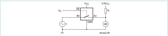
$Adjust \ f_i \ voltage \ to \ obtain \ 0 \ dBm \ level \ at \ output. \ Increase \ f_i \ frequency \ until \ dB \ meter \ reads \ -3 \ dB.$
