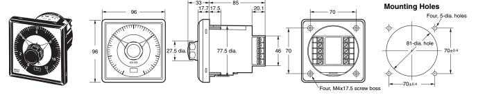
Note: Tightening torque for panel mounting is as follows: 0.3 N·m ±0.05 N·m
