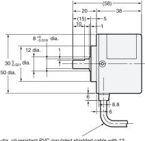
6-dia. oil-resistant PVC-insulated shielded cable with 12 conductors (Conductor cross section: 0.2 mm², Insulator diameter: 1.1 mm), Standard length: 1 m
