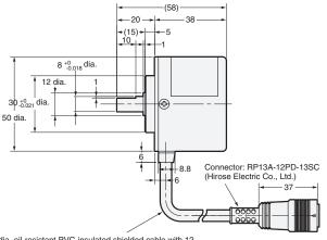
6-dia. oil-resistant PVC-insulated shielded cable with 12 conductors (Conductor cross section: 0.2 mm², Insulator diameter: 1.1 mm), Standard length: 1 m, Standard length for resolution of 360 or 720: 2 m
