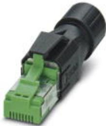
RJ45 connector, Degree of protection: IP20, Number of positions: 8, CAT5 (IEC 11801:2002), Material: PA 6.6, Connection method: IDC fast connection, Connection cross section: AWG 26-24, Cable exit: straight
