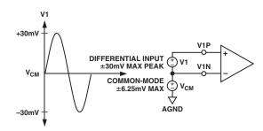
Figure 5. Maximum Signal Levels, Channel V1
