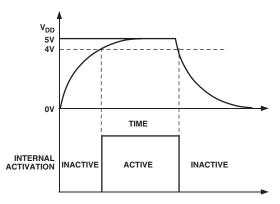
Figure 9. On-Chip Power Supply Monitor
