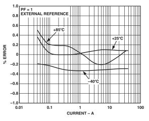
TPC 3. Error as a % of Reading over Temperature with External Reference (PF = 1)
