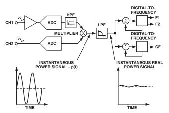
Figure 3. Signal Processing Block Diagram
