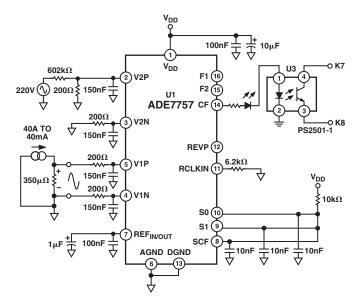
Figure 2. Test Circuit for Performance Curves
