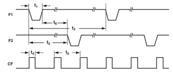
Figure 1. Timing Diagram for Frequency Outputs
