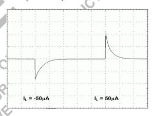
Figure 10. Load Transient Response
