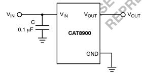
Figure 1. Application Circuit
