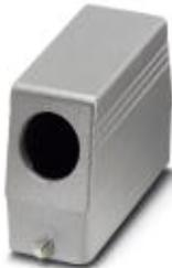
HEAVYCON sleeve housing B16, for single locking latch, height 76 mm, without support 1x M25, lateral conductor exit
