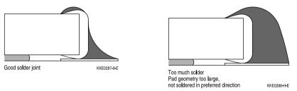
Good and poor solder joints caused by amount of solder in dual-wave soldering.
