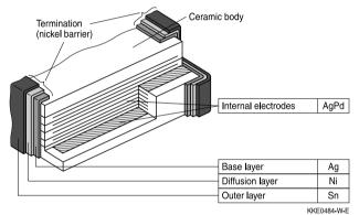
Multilayer CTVS: Structure of nickel barrier termination
