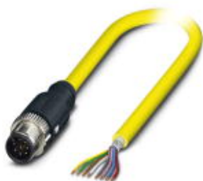
Sensor/actuator cable, 8-position, PVC, yellow, shielded, Plug straight M12 SPEEDCON, coding: A, on free cable end, cable length: 10 m
