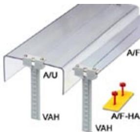
Flat-ribbon cover, for covering terminal strips, 2 mm thick, 9 cm wide, an additional requirement are 2 E/UK end brackets and 2 adjustable VAH cover holders. The max. supply length is 100 cm
