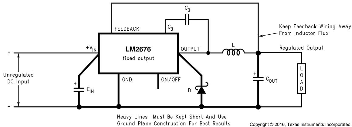
**Figure 21. Basic Circuit for Fixed Output Voltage Applications.**
