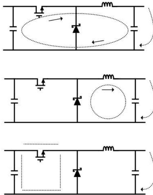
**Figure 23. Typical Current Flow on a Buck Converter**
