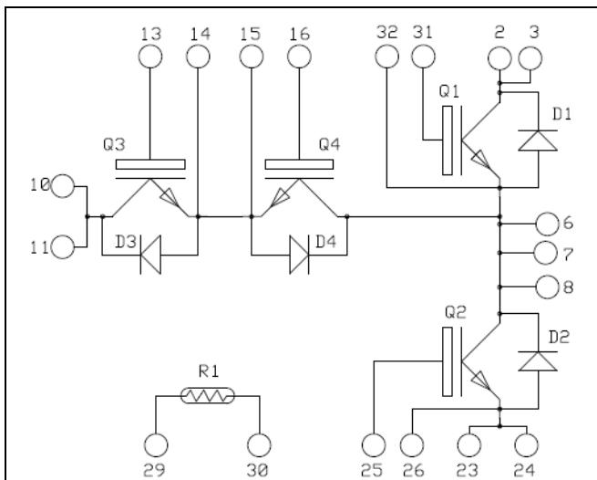
**High speed Trench & Field Stop IGBT4 (Q1, Q2):**
