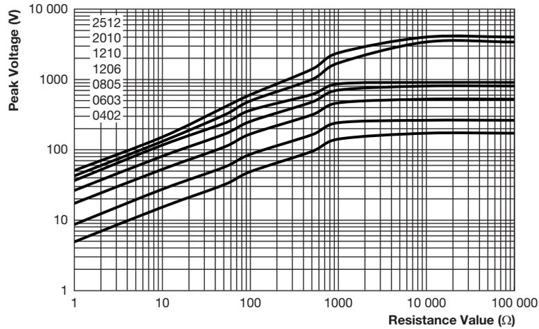
Pulse load rating in accordance to EN 60115-1, 4.27; 1.2  $\mu$ s/50  $\mu$ s;
