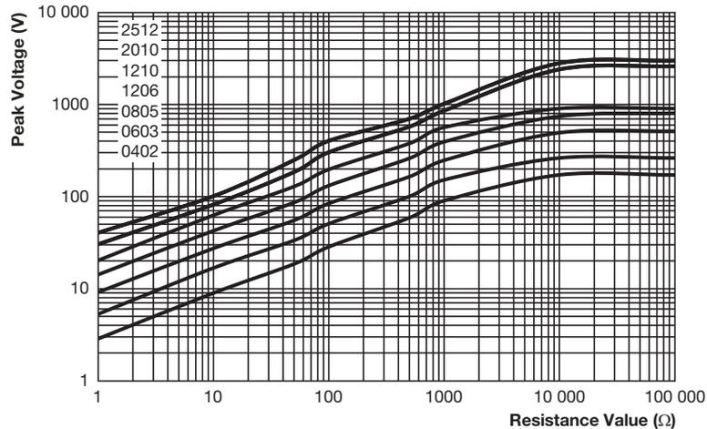
Pulse load rating in accordance to EN 60115-1, 4.27; 10  $\mu$ s/700  $\mu$ s;
