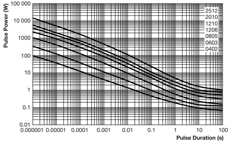
Maximum pulse load, single pulse; applicable if  $\bar{P} \rightarrow 0$  and  $n \leq 1000$  and  $\dot{U} \leq \dot{U}_{max}$ ; for permissible resistance change equivalent to 8000 h operation
