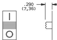
markings are reversed on V702 and V802 models. Actuator color is black with white markings (std.).
