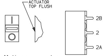
Markings are reversed on V702 and V802 models. Actuator color is red with white markings (std.). **Note:** Orientation of actuator markings and terminals.
