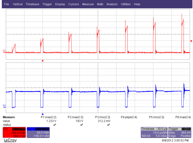
Figure 49 – 90 VAC, 60 Hz Start-up. Upper: I_{DRAIN} , 200 mA / div. Lower: V_{DRAIN} , 50 V, 10 \mu s / div.
