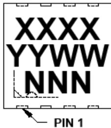
8-Lead DFN (3x3x0.9 mm) (MCP632)
