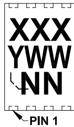
8-Lead DFN (3x3x0.9 mm) (MCP632)
