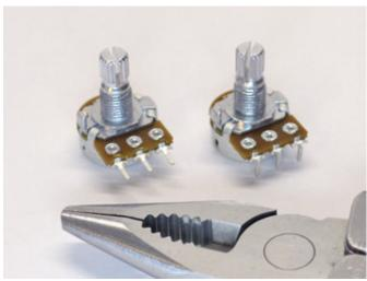
If adding more than one potentiometer, the legs must be bent back to fit inside the case. If two potentiometers are installed in the same quadrant, they install back-toback.
