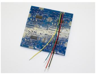
Looking at the back of the tiled Trellis boards...with the text upright, in the normal orientation for reading... connect the wires to the header along the **top edge**, toward the **right**. They should be about 6 inches (15 cm) long, or a little longer.
