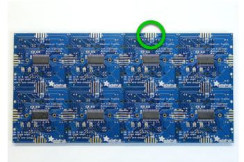
On the HELLA UNTZtrument — a 4x2 assembly of Trellises — connect the wires to the third header along the top edge, not the rightmost fourth header.
