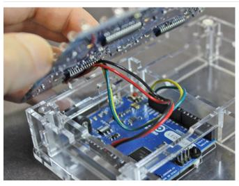
Now the Trellis gets turned over, LED side up, and is lowered into place in the case. You'll see the horizontal and vertical braces have notches into which the board neatly fits.
