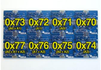
Here's the address map for the HELLA UNTZtrument.
