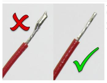
When tinning stranded wires (to prevent fraying and shorts), use just a *tiny bit* of solder, and make sure it *fully flows* into the strands. Sometimes you'll want to clip off the very tip of the wire if the iron left a glop or spike there.
