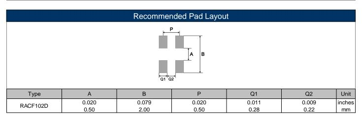
Concave Termination Chip Resistor Array
