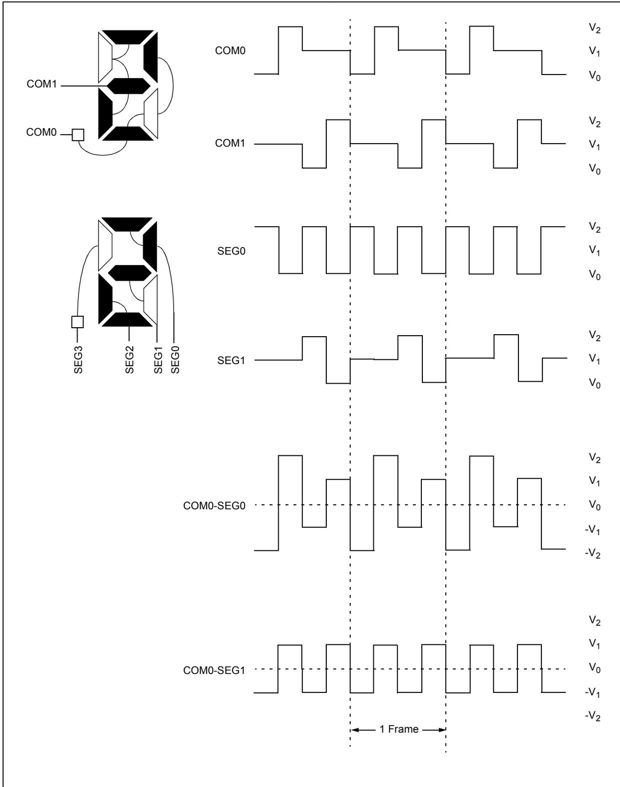
**FIGURE 22-6: TYPE-B WAVEFORMS IN 1/2 MUX, 1/2 BIAS DRIVE**
