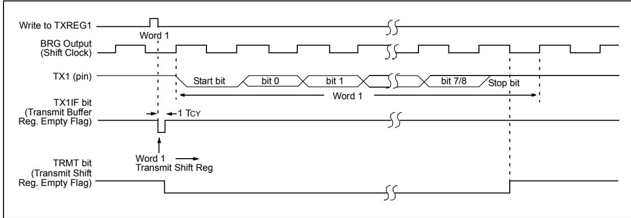
**FIGURE 16-5: ASYNCHRONOUS TRANSMISSION (BACK-TO-BACK)**
