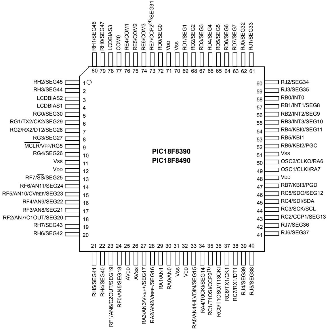
**Note 1:** RE7 is the alternate pin for CCP2 multiplexing.
