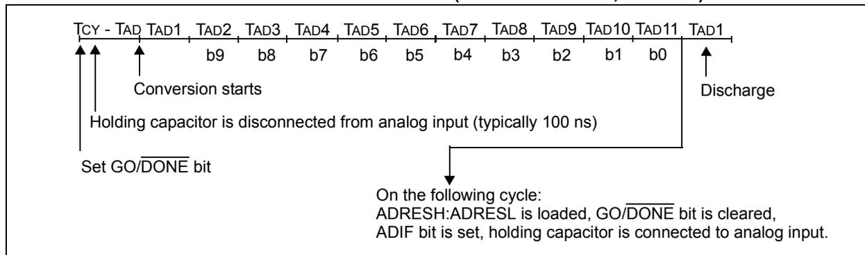
**FIGURE 18-5: A/D CONVERSION TAD CYCLES (ACQT<2:0> = 010, TACQ = 4 TAD)**
