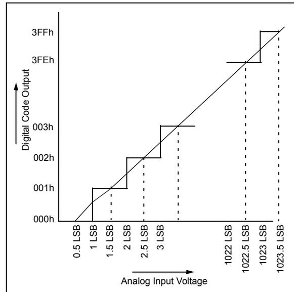
**FIGURE 18-3: ANALOG INPUT MODEL**
