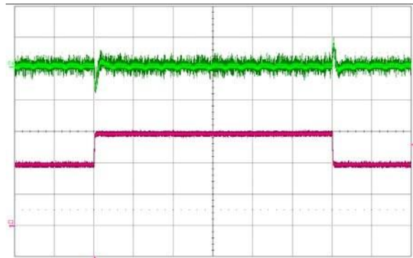
Figure 12. Output voltage response to load current step change (10 A – 15 A – 10 A) at V_{in} = 48 V. Top trace: output voltage (100 mV/div.) Bottom: load current (5 A/div.). Current slew rate: 1 A/μs. Time scale: 200 μs/div. C_o = 470 μF POS + 1 μF ceramic
