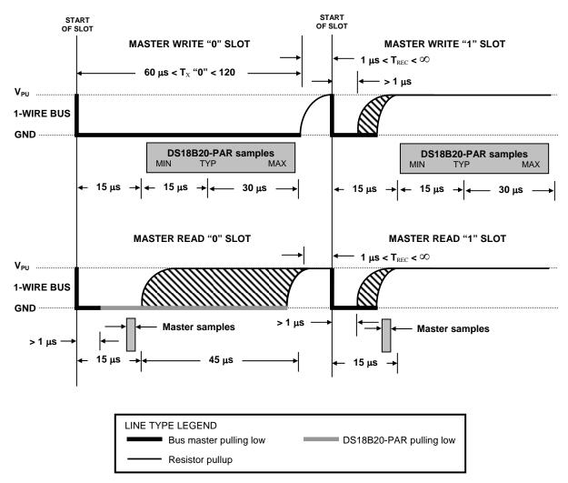
**READ/WRITE TIME SLOT TIMING DIAGRAM** Figure 13
