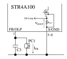
Figure 9-5. FB/OLP Pin Peripheral Circuit
