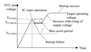
Figure 9-3. VCC Pin Voltage During Startup Period
