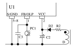
Figure 9-10. FB/OLP Pin Peripheral Circuit
