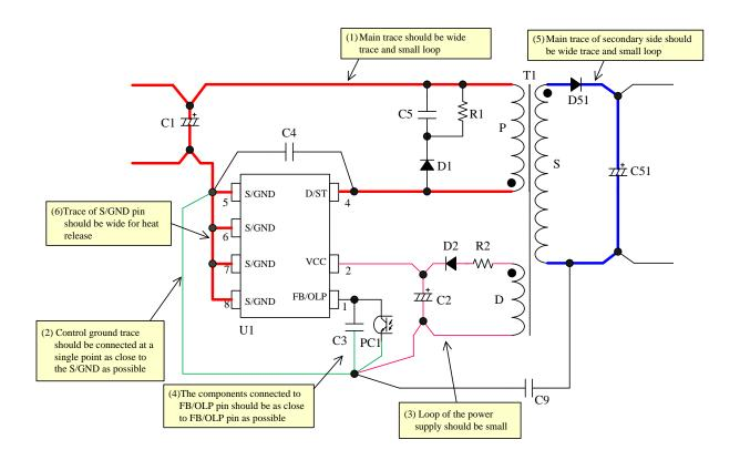
Figure 10-7. Peripheral Circuit Example Around IC
