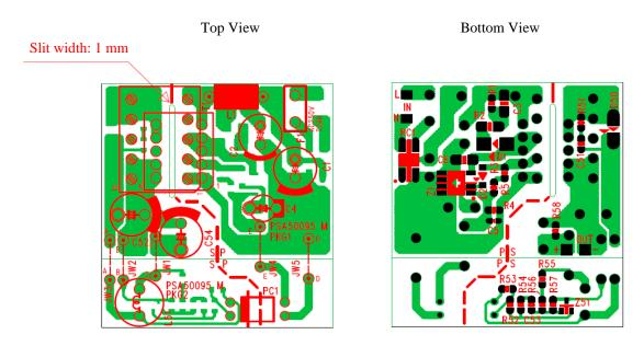
Figure 11-1. PCB Layout Example (SOIC8 Type)
