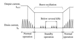
Figure 9-8. Auto-standby Mode Timing
