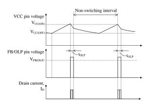
Figure 9-11. OLP Operational Waveforms
