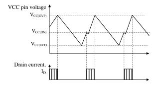
Figure 9-12. OVP Operational Waveforms
