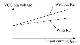
Figure 10-2. Variation of VCC Pin Voltage and Power
