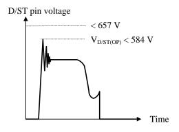
Figure 10-4. D/ST Pin Voltage Waveform in Normal Operation
