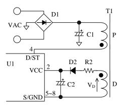
Figure 9-1. VCC Pin Peripheral Circuit
