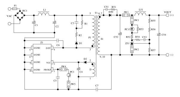
Figure 11-2. Circuit Schematic for PCB Layout
