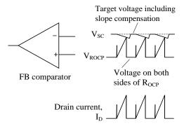
Figure 9-6. Drain Current, I<sub>D</sub>, and FB Comparator Operation in Steady Operation
