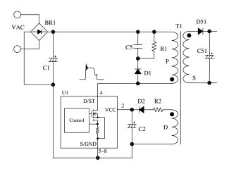
Figure 10-3. D/ST Pin Peripheral Circuit
