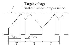
Figure 9-7. Drain Current, I<sub>D</sub>, Waveform in Subharmonic Oscillation
