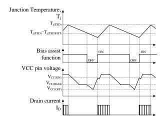
Figure 9-14. TSD Operational Waveforms
