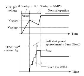
Figure 9-4. V<sub>CC</sub> and I<sub>D</sub> Behavior During Startup
