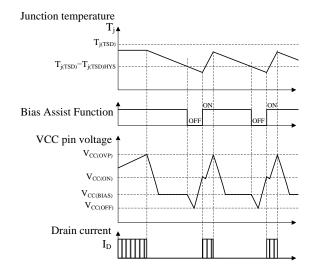
Figure 9-13. OVP Operational Waveforms in High Temperature
