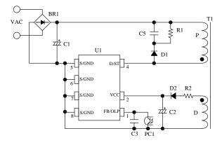
Figure 10-1. IC Peripheral Circuit
