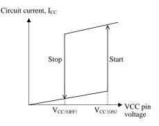
Figure 9-2. Relationship between VCC Pin Voltage and I<sub>CC</sub>
