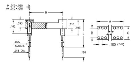
**Description:** DIP Dual In Line Socket Pluggable Wrapost Tail Open Frame Through Hole Plating Code: Shell Plating: 200 μ" Tin/Lead(93/7) over 100 μ" Nickel Inner Contact Plating: 10 μ" Gold over 50 μ" Nickel Packaging: Packaged in Tubes
