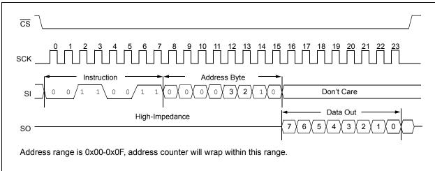
To write to the unique ID locations, the IDWRITE command is used. The device must be write enabled and the correct unlock sequence must have been performed. See Section 10.1.4, Write to the Unlock Register for more details.
