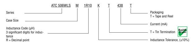
The above part number refers to a 506WLS Series, Case Size M, 1.10 µH inductor, K tolerance (±10%, typ.), with Tin Termination (T), 438 mA, tape and reel packaging.
