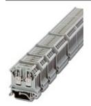
Basic termination blocks with screw connection for NS 32 and NS 35/7.5 DIN rail, with end cover, for ST-REL..., ST-OV... and ST-OE... plugs, 7-pos.
