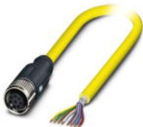
Sensor/actuator cable, 8-position, PVC, yellow, shielded, free cable end, on Socket straight M12 SPEEDCON, A-coded, cable length: 10 m
