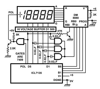
FIGURE 8. ICL7135 PLASMA DISPLAY CIRCUIT
