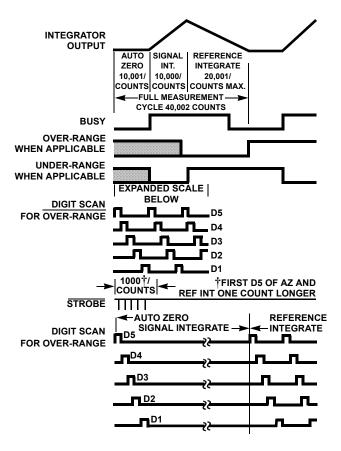
FIGURE 6. TIMING DIAGRAM FOR OUTPUTS
