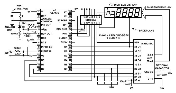
FIGURE 10. DRIVING LCD DISPLAYS
