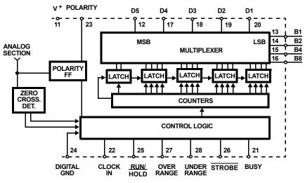
FIGURE 5. DIGITAL SECTION OF THE ICL7135
