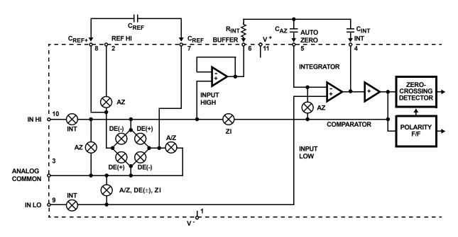
FIGURE 3. ANALOG SECTION OF ICL7135
