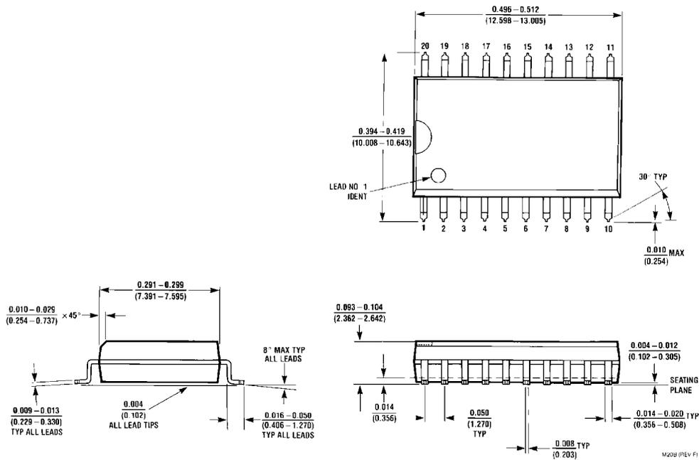
**20-Lead Small Outline Integrated Circuit (SOIC), JEDEC MS-013, 0.300" Wide Body
