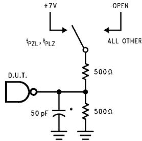
\*Includes jig and probe capacitance
