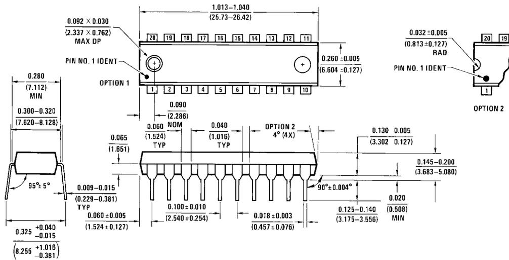
**20-Lead Plastic Dual-In-Line Package (PDIP), JEDEC MS-001, 0.300" Wide
