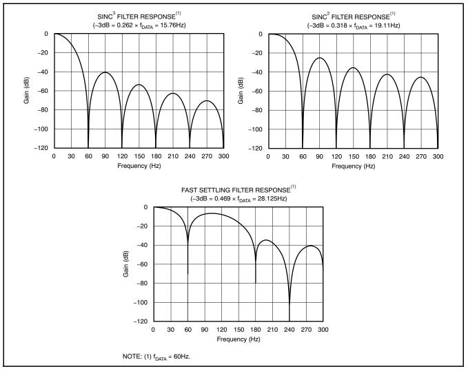
Figure 28. Filter Frequency Responses
