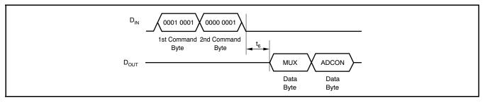
Figure 34. RREG Command Example: Read Two Registers Starting from Regiater 01h (multiplexer)
