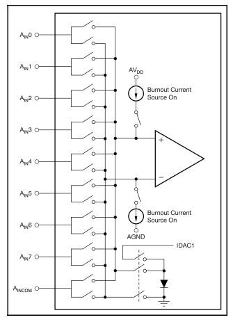
Figure 25. Input Multiplexer Configuration
