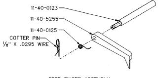
FEED FINGER ASSEMBLY FOR PRESS \*TM40
