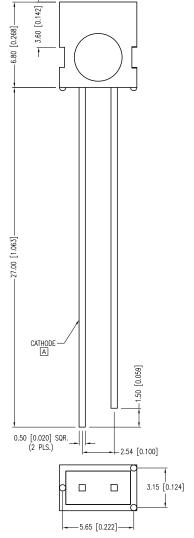
\*UNLESS OTHERWISE SPECIFIED TOLERANCES PER DECIMAL PRECISION ARE: X=±1 (±0.039), XX=±0.5 (±0.020), XXX=±0.25 (±0.010), XXXX=±0.127 (±0.005). LEAD SIZE=±0.05 (±0.002), LEAD LENGTH=±0.75 (±0.030). MIN=  $\frac{+0.00}{-0.00}$  MAX.=  $\frac{+0.00}{-0.00}$  MAX
