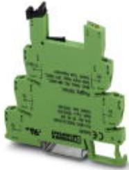
6.2 mm PLC basic terminal block with spring-cage connection, without relay or solid-state relay, for mounting on DIN rail NS 35/7,5, 1 PDT, input voltage 230 V AC/DC
