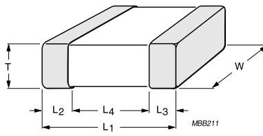
Fig. 2 Surface mounted multilayer ceramic c
