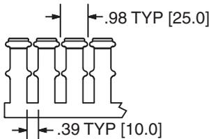
Multiple slot restrictors present with 75mm and greater duct wall height.
