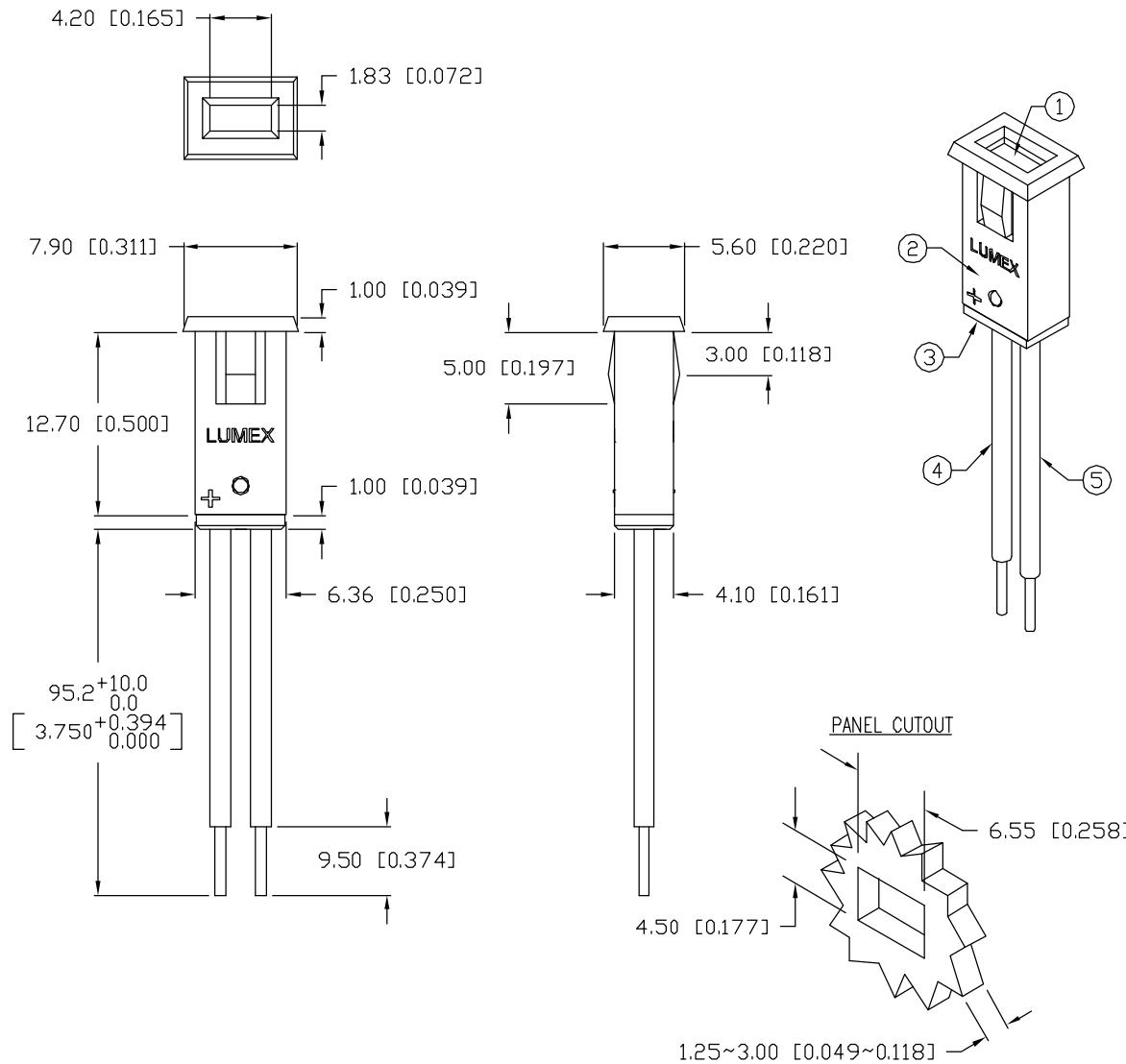
\*UNLESS OTHERWISE SPECIFIED TOLERANCES PER DECIMAL PRECISION ARE: X=±1 ( $\pm 0.039$ ), X.X=±0.5 ( $\pm 0.020$ ), X.XX=±0.25 ( $\pm 0.010$ ), X.XXX=±0.127 ( $\pm 0.005$ ). LEAD SIZE=±0.05 ( $\pm 0.002$ ), LEAD LENGTH=±0.75 ( $\pm 0.030$ ). MIN=  $^{+0.00}$  MAX=  $^{+0.00}$  DECIMAL PRECISION
