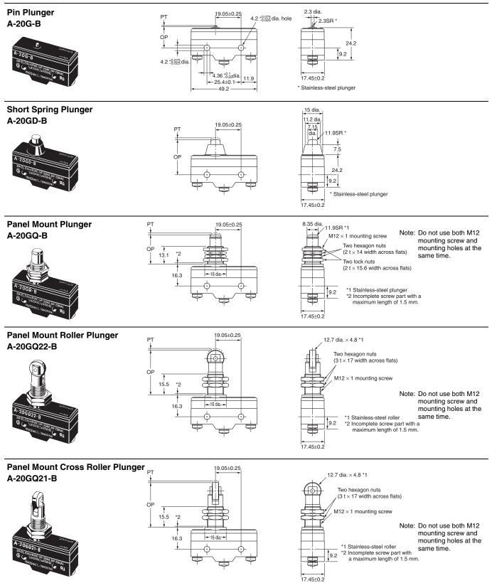
Note: Unless otherwise specified, a tolerance of  $\pm 0.4~\text{mm}$  applies to all dimensions.
