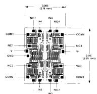
NOTE: NCx IS CONNECTED TO COMx WHEN INX IS LOW.
