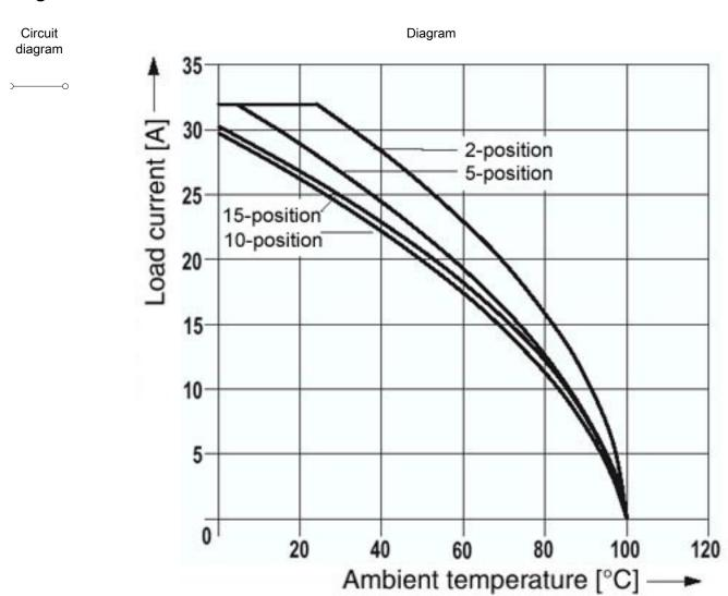
Derating curve for the spring-cage terminal with all plug versions SP  $4/\dots$
