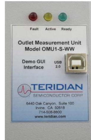
Alternatively, the user can directly query the device with the command set using HyperTerminal and the provided *6612\_OMU\_S2\_URT\_V1\_13 Firmware Description Document*.
