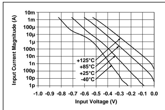
**FIGURE 2-42:** Input Bias Current vs. Input Voltage.
