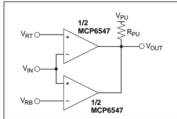
FIGURE 4-10: Windowed Comparator.
