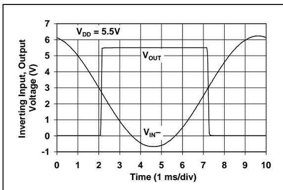
**FIGURE 2-3:** The MCP6546/6R/6U/7/8/9 Comparators Show No Phase Reversal.
