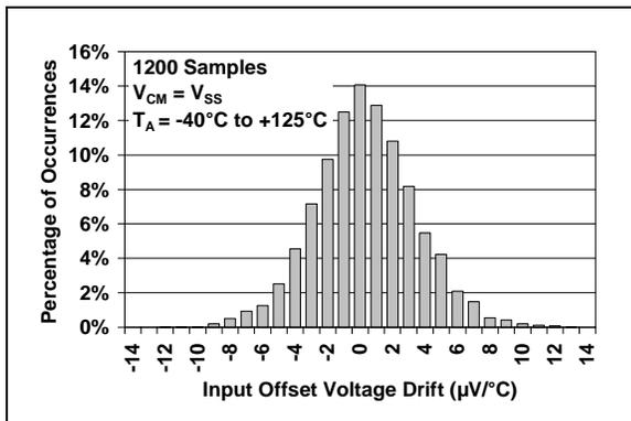
**FIGURE 2-2:** Input Offset Voltage Drift at  $V_{CM} = V_{SS}$ .
