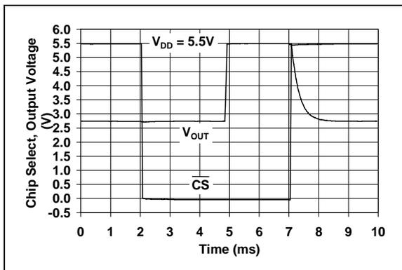
**FIGURE 2-39:** Chip Select (CS) Step Response (MCP6548 only).
