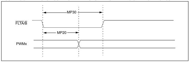
FIGURE 26-10: MOTOR CONTROL PWM MODULE TIMING CHARACTERISTICS
