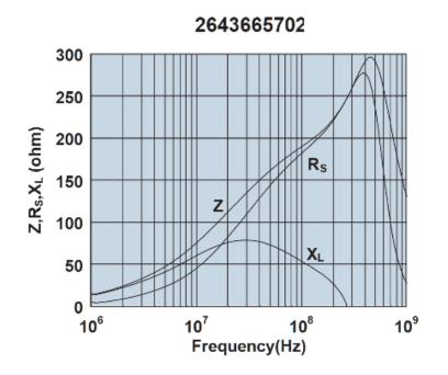
Impedance, reactance, and resistance vs. frequency.
