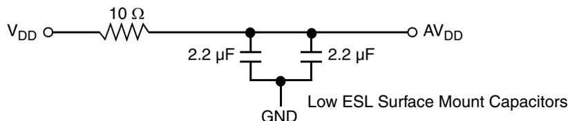
**Figure 75. Chip PLL Power Supply Filter Circuit**
