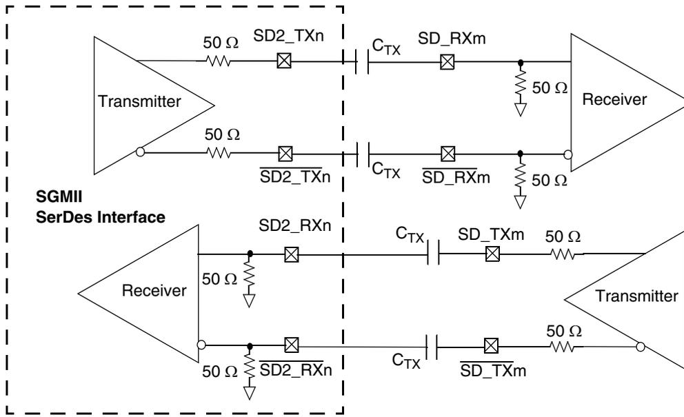
Figure 29. 4-Wire AC-Coupled SGMII Serial Link Connection Example
