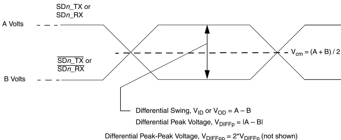
**Figure 57. Differential Voltage Definitions for Transmitter or Receiver**
