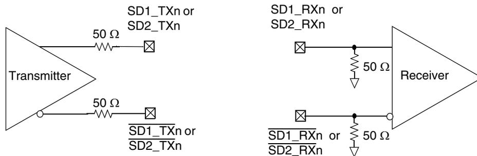
**Figure 68. SerDes Transmitter and Receiver Reference Circuits**
