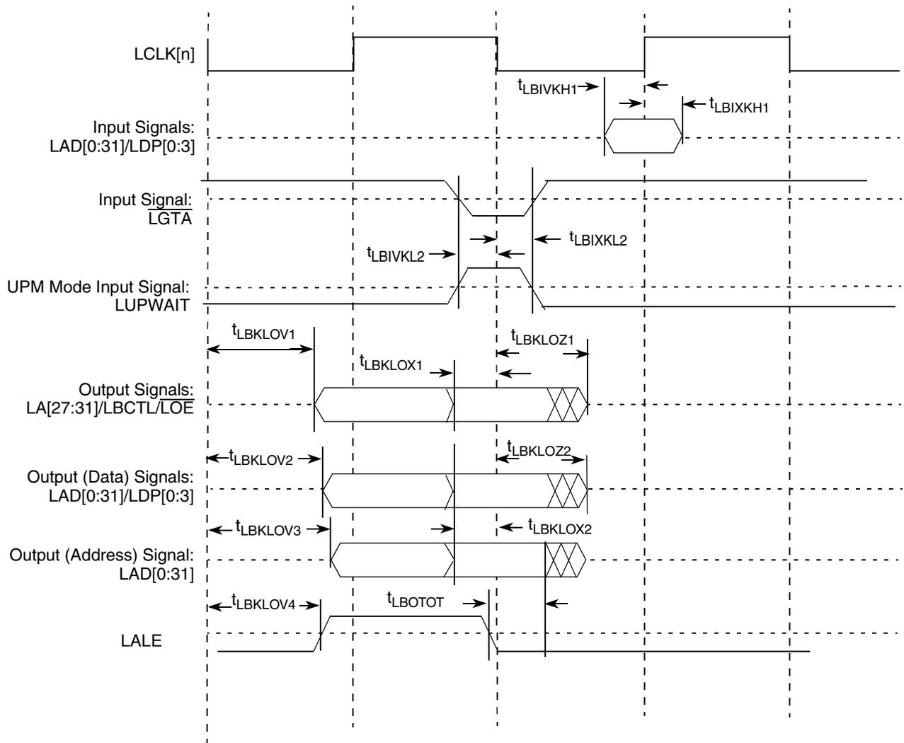
Figure 40. Local Bus Signals (PLL Bypass Mode)
