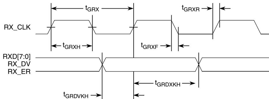
Figure 18. GMII Receive AC Timing Diagram
