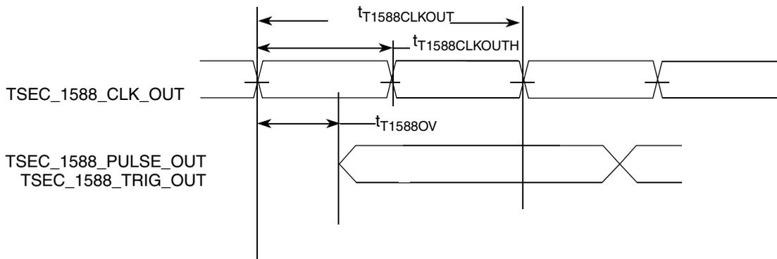
Figure 33. eTSEC IEEE 1588 Output AC timing
