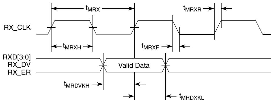
Figure 21. MII Receive AC Timing Diagram
