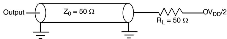
**Figure 45. AC Test Load for the JTAG Interface**
