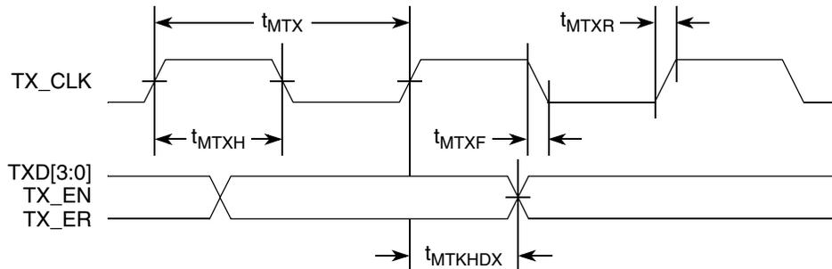
Figure 19. MII Transmit AC Timing Diagram
