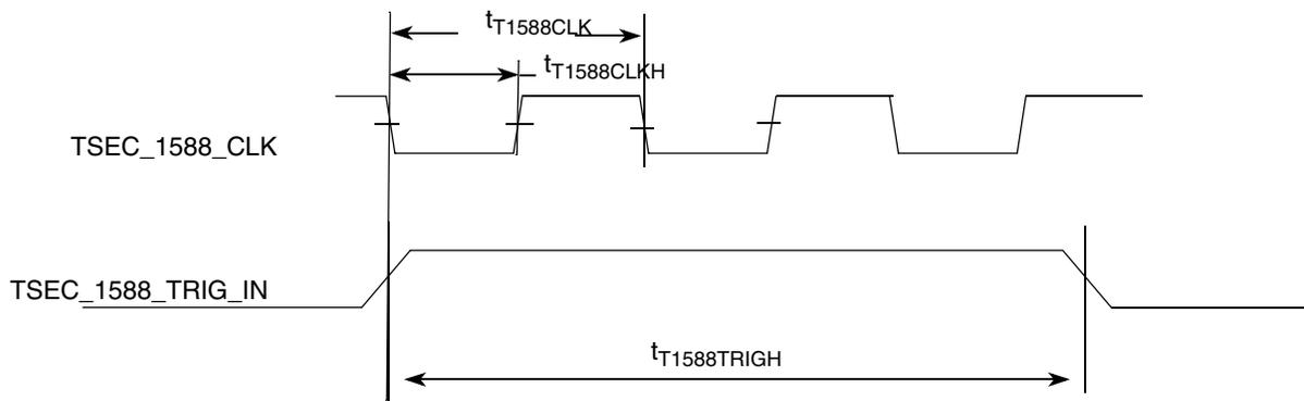
Figure 34. eTSEC IEEE 1588 Input AC timing
