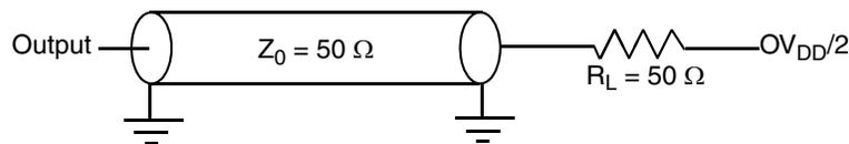
**Figure 51. I<sup>2</sup>C AC Test Load**
