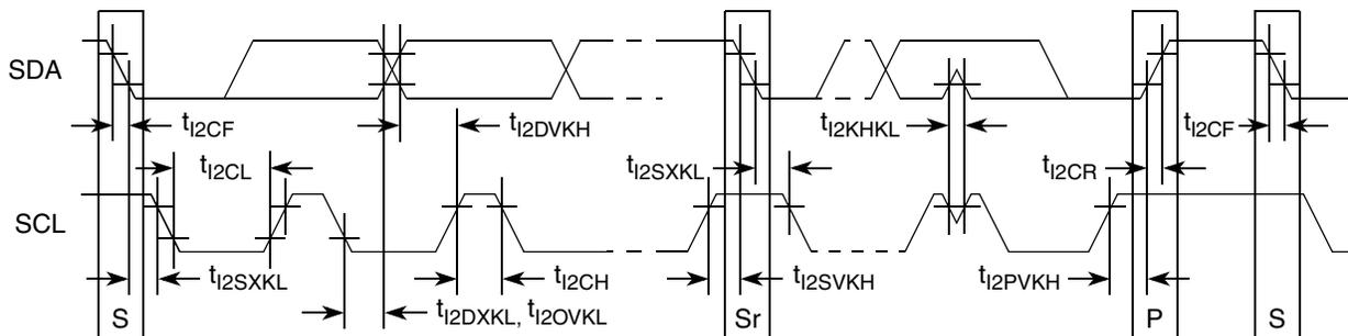
**Figure 52. I<sup>2</sup>C Bus AC Timing Diagram**
