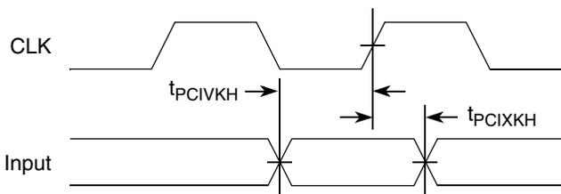
**Figure 55. PCI Input AC Timing Measurement Conditions**
