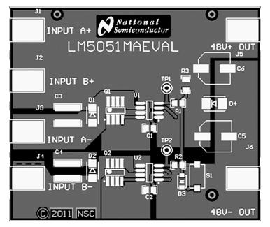
Figure 9. Evaluation Board, Top Side (Component)
