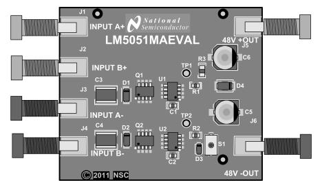
**Figure 8. Component Placement**
