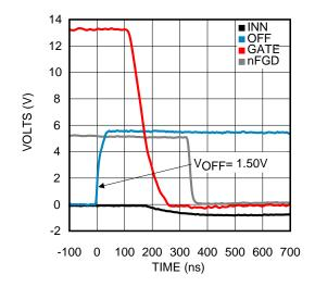
Figure 4. OFF pin Going High, Gate OFF
