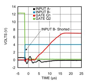
Figure 2. Forward and Reverse Waveforms
