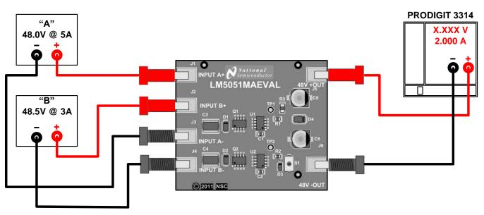
**Figure 1. Typical Board Connections**
