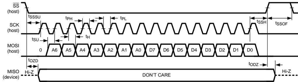
Figure 4. SPI Write
