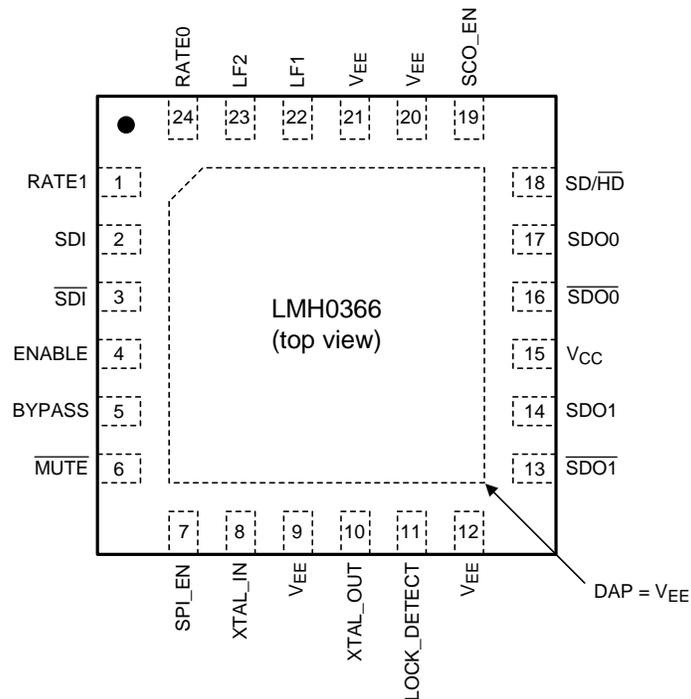
Figure 1. Pin Mode (non-SPI) / SPI\_EN = GND
