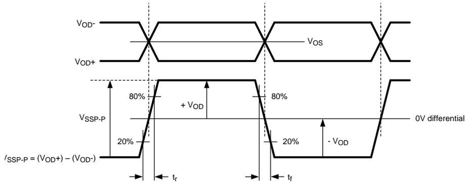
Figure 3. LVDS Output Voltage, Offset, and Timing Parameters
