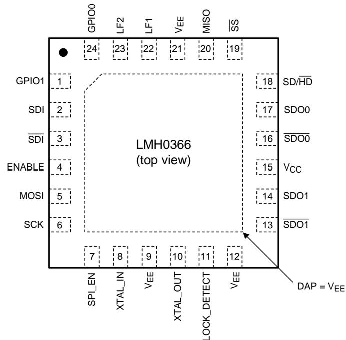
The exposed die attach pad is the primary negative electrical terminal for this device. It must be connected to the negative power supply voltage.
