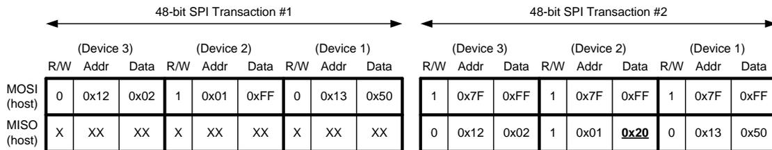
Figure 9. SPI Daisy-Chain Read and Write Example
